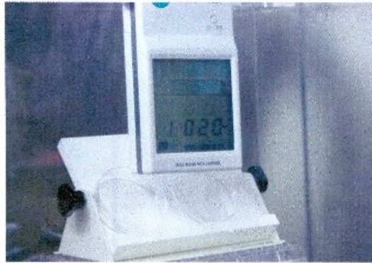
Photo 2: Measurement of ion concentration by ion counter.
